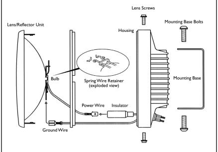
Use this illustration when changing the bulb or repositioning the bracket for correct mounting.
